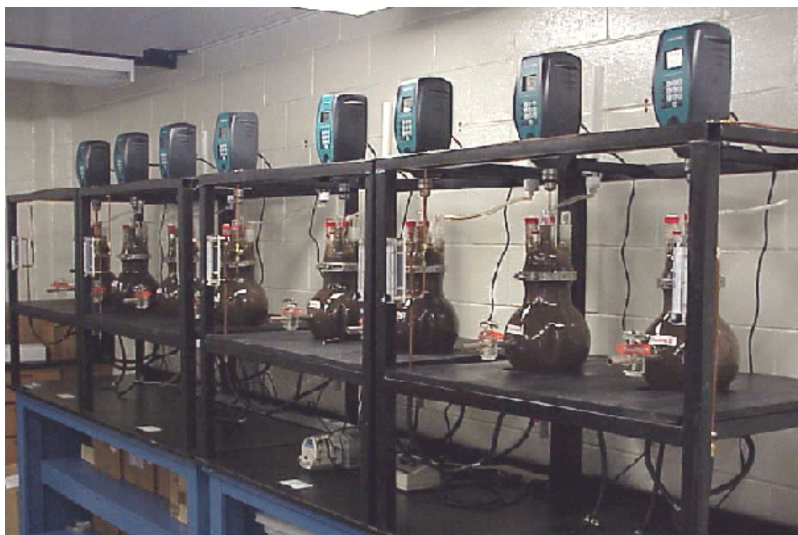
Figure 4.2. Photograph of the Bioslurry Reactor Setup
